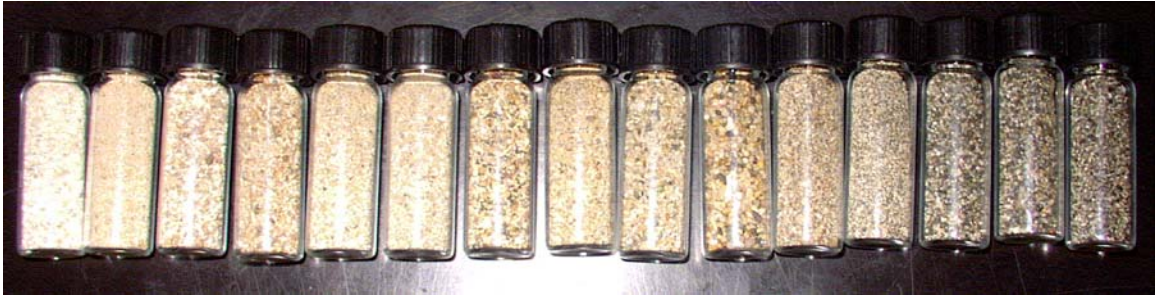
Figure 7: Sand of the 15 beaches, the order corresponds to the magnitude of the measurement with the GER 1500 from high (left) to low (right).
